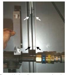
Figure 10. Install rear connecting plate.
